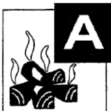
Flammable solids and those form flames or smoulder
